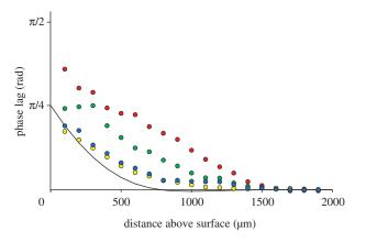
Figure 5. Observed phase lag between the far-field and local flow for two MEMS hairs as a function of interhair distance (red 600  $\mu$ m, green 1000  $\mu$ m, blue 1700  $\mu$ m and yellow 2800  $\mu$ m) at the flow frequency of 80 Hz. The solid line represents the expected phase lag on a flat plate, given in equation (2.4).
