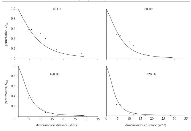
Figure 4. Flow perturbation between two MEMS hairs, as a function of interhair distance and flow frequency. Filled circles represent measurements while lines represent predicted data from the analytical model (equation (2.6)). The distance between the two hairs is denoted by s and the hair diameter by d.
