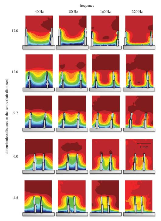
Figure 3. Full-field data for flow in the vicinity of MEMS hairs arranged in tandem, as a function of frequency and interhair distance. Data for the largest interhair distance are not shown owing to the need for different scaling.
