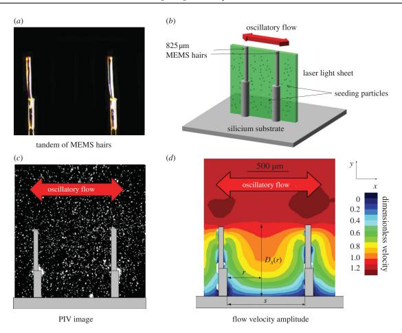
Figure 1. Set-up and definition of variables.
